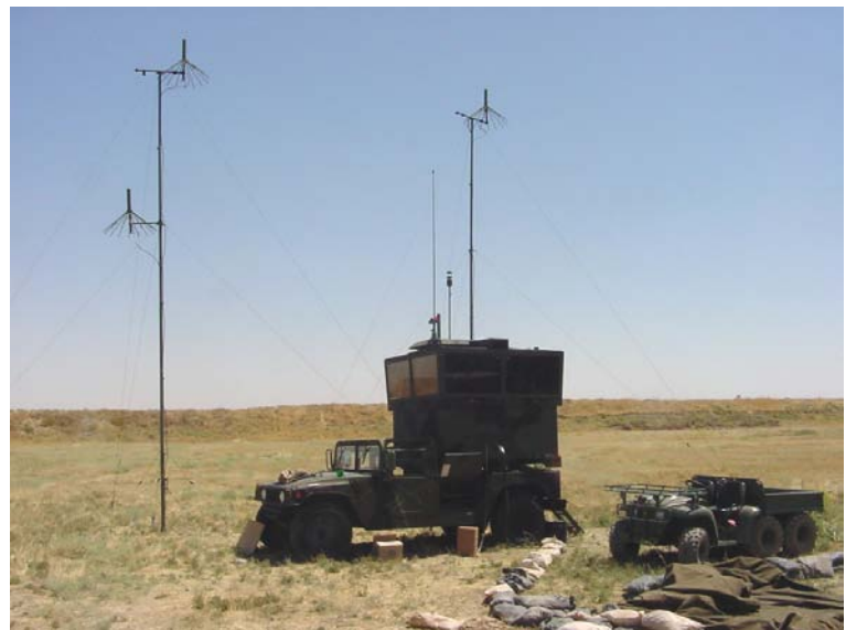
Remote Landing Site Tower (AN/TSQ-216) in Operation
